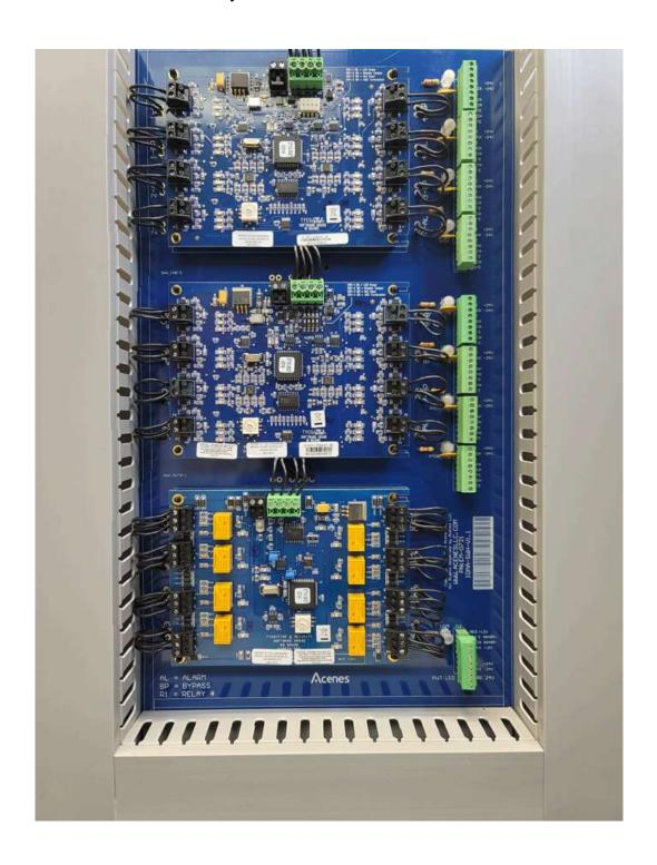
All the installer needs to do is bring one 8-Conductor wire to the STB-IDMA-SWH Termination Board for it to communicate with the Software House Access Control System.
